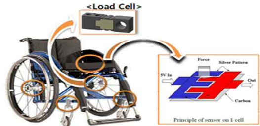
Figure 3. Load cell installation(left), Pressure sensor installation(right)
