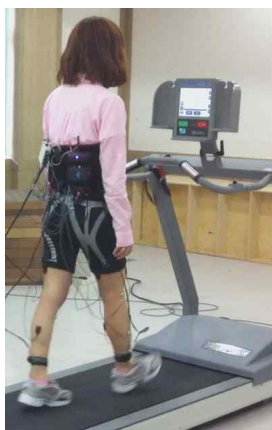
Figure 2. EMG and plantar pressure measurement during walking on treadmill
