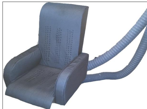
Figure 1. Chair applied air conditioning systems
