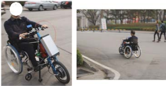
Figure 7. Drivability Test of Manual Wheelchair with Drive-assisting System Prototype
