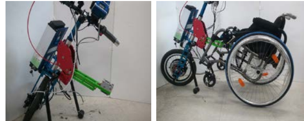
Figure 5. Prototype of Driving-Assisting System available for Manual Wheelchair
