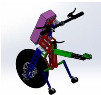
Figure 3. Finalized 3D Design of Drive-assisting System with Battery and Brake Mechanism
