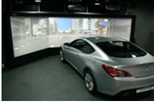
Figure 1. Driving Simulator for Human-in-the-Loop Experiment
