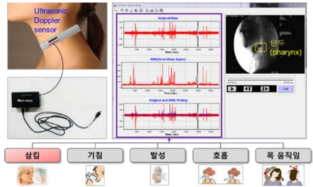
Figure 3. Laryngopharyngeal movements measured by the swallowing measurement device (Lee et al., 2012)
